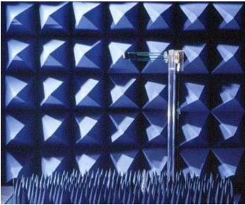
Antenna Setup in CTIA 3D Chamber
