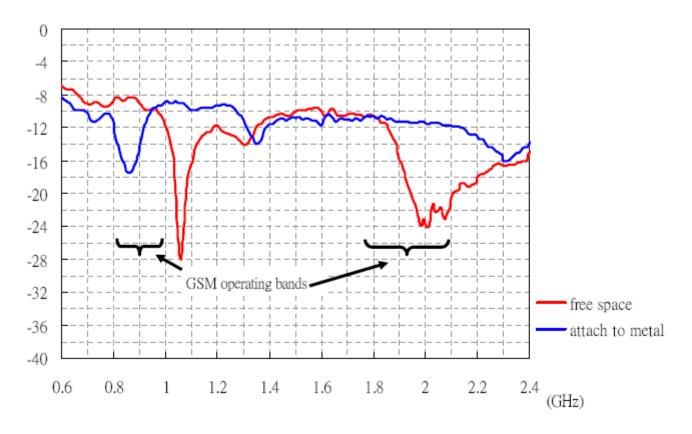
**GSA.8821** Return Loss in Free Space and adhered to Metal. The oscillation introduced by the 3m cable is smoothed with a factor of 1%.
